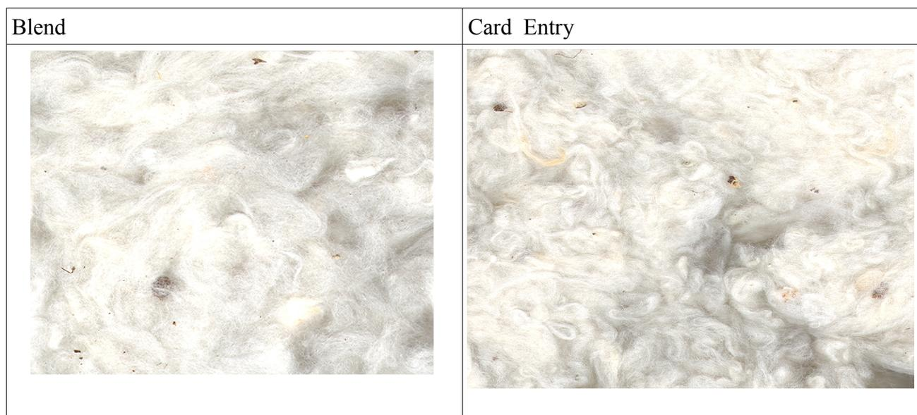
Tearing of fibers before card entry caused by harsh cleaning in blow room .
